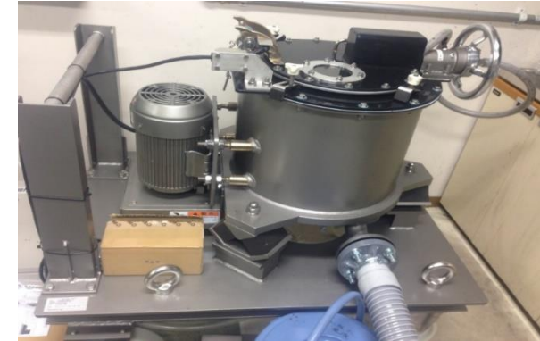
Continuous centrifugation (12 L) >500 g / batch
